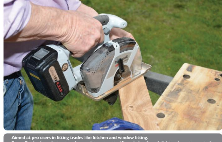
Pros:- Dual voltage battery pack capacity, cuts up to 43mm in hardwood, light and easy to control with good dust extraction.
